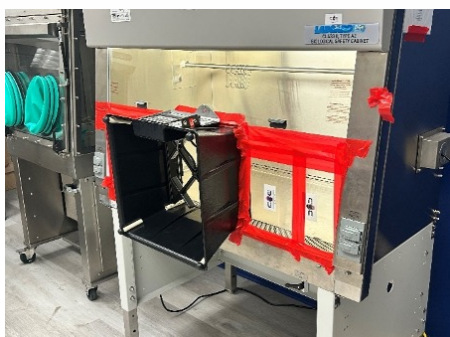
The three flow hood configurations used in this experiment, as well as the method they were connected to the biosafety cabinet.
