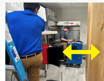
How the obstruction was used to simulate various distances between the front intake opening and a wall. The yellow arrow represents where the corresponding distance was measured.
